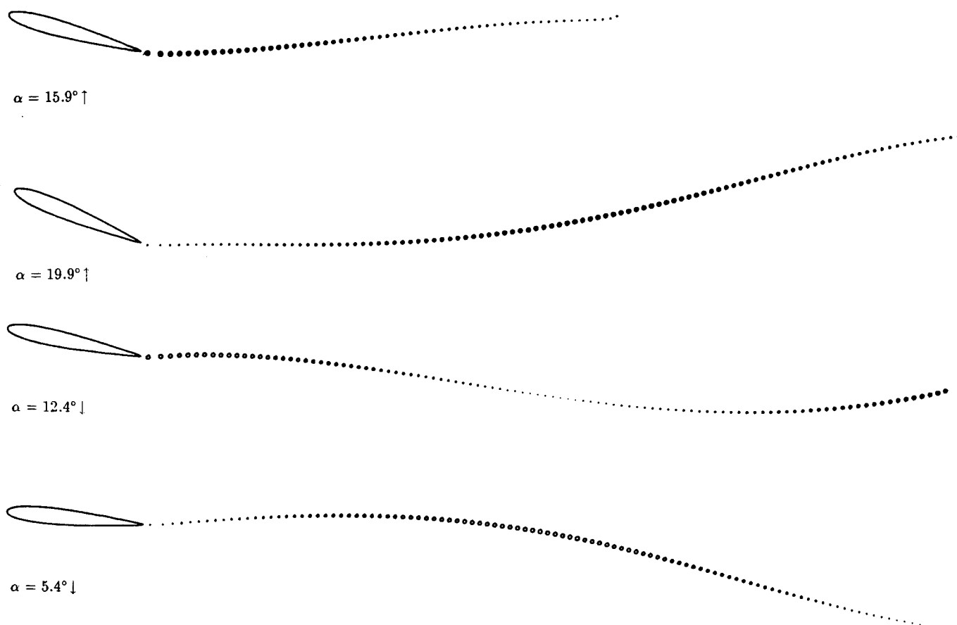
Fig. 13 Instantaneous locations of wake vortex filaments: \alpha_{\min} = 0 deg, \alpha_{\max} = 20 deg, and k = 0.25 .
